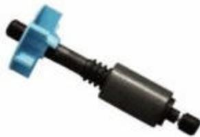
If you just take the time about every 3 months to remove and clean the impeller assembly and impeller housing (the area where the impeller spins), you will remove slime accumulation, debris, sand, grit and calcareous build-up (in saltwater tanks) thus reducing friction in the motor housing. This will increase the water flow of the filter or pump and ensure that the unit starts right back up after the power has been turned off. What damages these types of motors
