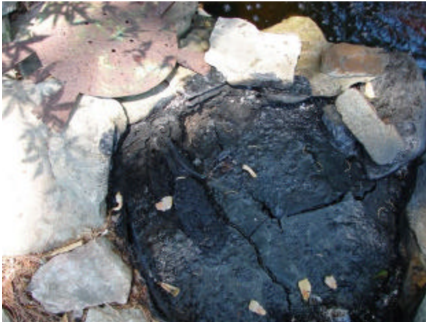
THE REMAINS OF A SAVIO SKIMMER IN THE SUMMERVILLE AREA AFTER THE UV CAUGHT FIRE AND MELTED THE ENTIRE UNIT.....
